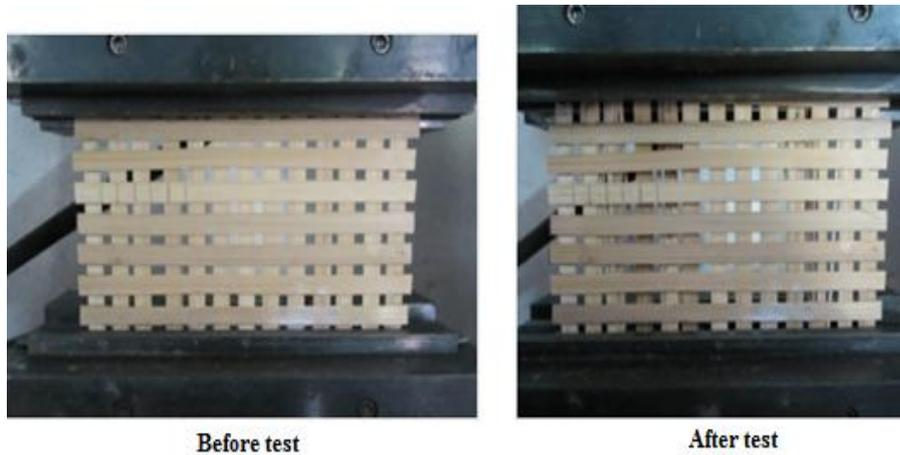
**Figure 1: Wide Width Tensile Strength Test on a Bamboo Geogrid Specimen**
