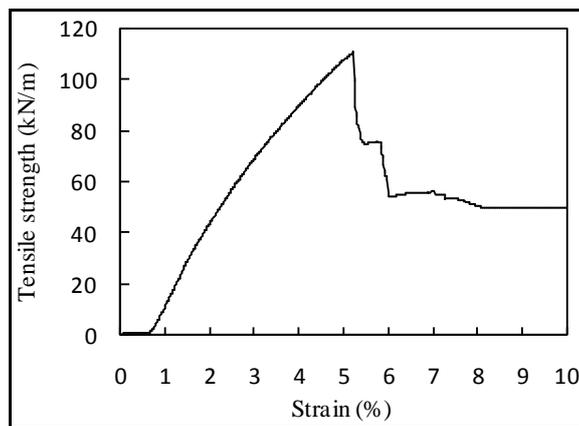
**Figure 2: Tensile Strength-Strain Behaviour of Bamboo Geogrid**
